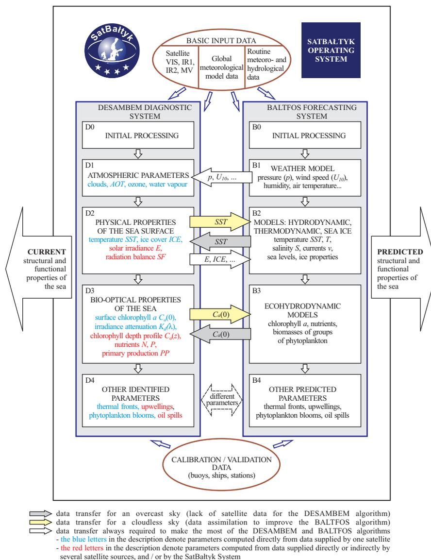
**Figure 2.** Block diagram of the SatBałtyk Operational System
